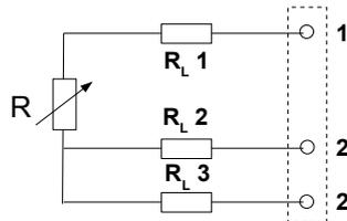
This connection involves identical line resistors (RL1-RL2-RL3), RL2 + RL3 allow you to measure the line resistance that will be subtracted from the measured resistance between 1 and 22' terminals. This is the most common connection.
