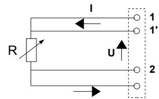
Regulated current is going through 11' and 22' terminals and the measurement is made at the sensor terminals, so none of the line resistors are taken into account. This is the most accurate connection.
